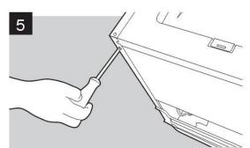
Remove the screw from the side of the Larder Fridge where the bracket is to be re-fitted and replace on the other side.
